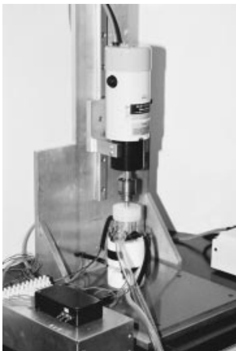
Shown above is a bench-scale UV reactor.
