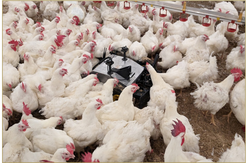
ATRP researchers are field testing an autonomous mobile robot in a push to demonstrate its commercial readiness. The robotic assistant is designed to perform management tasks in commercial poultry houses with the goal of reducing labor while potentially mitigating disease and contamination factors.
